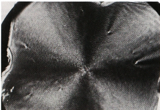
Figure 5 PBLG film prepared with cylindrical rotating cap. Concentration 13.5%; solvent dioxane 1 ; diameter 20 mm; 2000 rev min -1 clockwise; crossed polarizers; angle of the polarizer axes 12 h, 3 h
